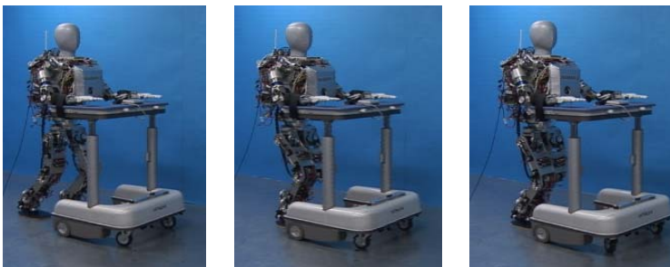
Fig. 4. WABIAN-2 using the Walking Support Device
