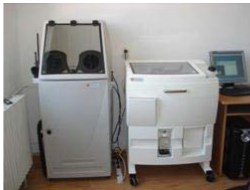
Fig. 71. Rapid prototyping device - 3D printer
