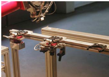
Fig. 2. Quality monitoring of aircraft fuselages with wide- and short-range inspection sensors. Left: Inspection station and test environment. The movement of production pieces is carried out by monorail conveyors which do not allow precise positioning. Right: Development and demonstration platform (DDP).
