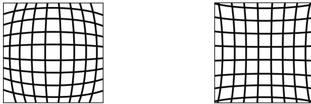
Fig. 9. The left pattern depicts the effect of radial distortion, whereas the right pattern shows the effect of tangential distortion.
